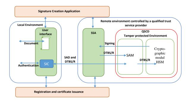
Type 2 QSCD is a combination of a cryptographic module and a SAM. The relevant security requirements are set out in the following Protection Profiles (PP) issued as European Standards:
